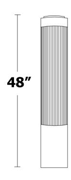
Steel Pipe ID = 10" Steel Pipe OD = 10.75" Ideal Sleeve ID = 10 7/8"
